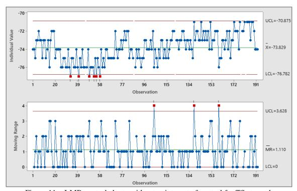
Figure 11 – I-MR control charts without points out of control for TS strength
