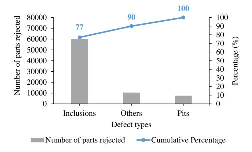
Figure 4 – Pareto chart for the number of parts rejected during the month of April through September 2019. Source: Internal data of Fehst Componentes, Lda, 2019.
