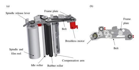
Figure 3 - 3D CAD model of the pre-stretching device: (a) front view and (b) top view, with indication of the main components.
