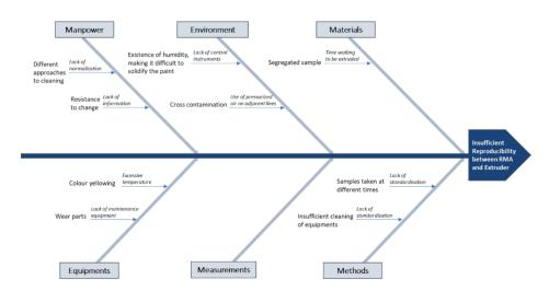
Figure 18 - Ishikawa Diagram to analyse the insufficient reproducibility between RMA and extruder
