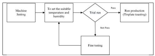
Figure 4. ABC operation flow of tinplate toasting
