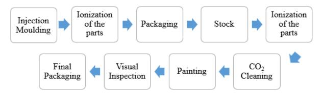
Figure 1 – Manufacture steps of the High Gloss Blend parts.
