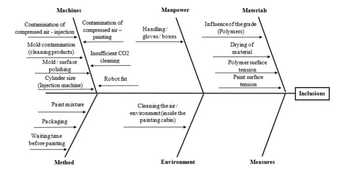
Figure 5 – Ishikawa diagram for the inclusion defect (Elaborated by the authors).
