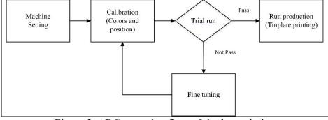
Figure 3. ABC operation flow of tinplate printing
