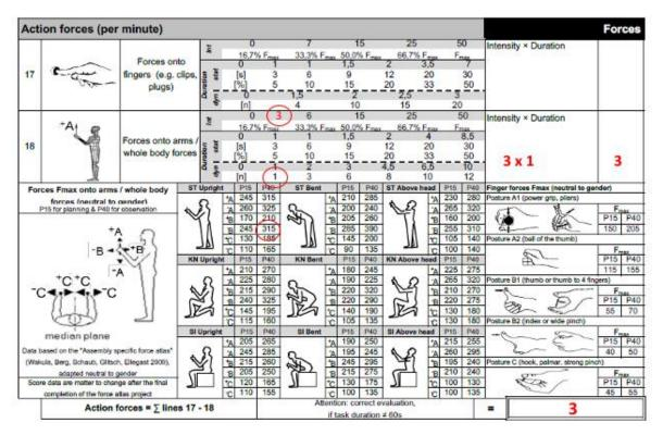
Figure 4 – Action forces section of EAWS. Evaluations for the task are provided in red.
