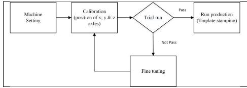
Figure 5. ABC operation flow of tinplate stamping
