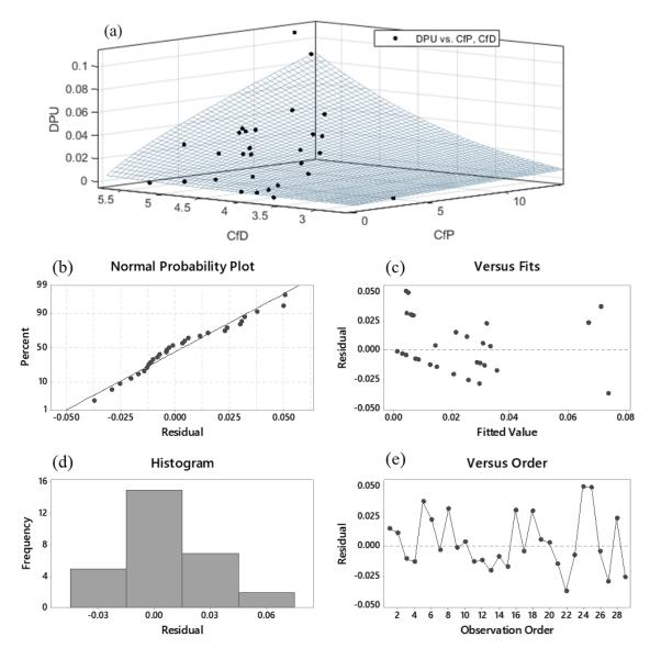
Figure 7 - (a) DPU vs  $Cf_P$  and  $Cf_D$ : defect prediction model, see Eq. (5), and experimental data; Plots of residuals between nominal DPU and predicted DPU: (b) Normal Probability Plot, (c) Residuals vs Fitted values, (d) Histogram and (e) Residuals vs Order.
