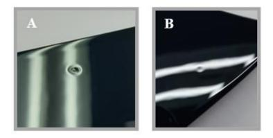
Figure 3 – Main part defects detected by the sensor: (A) Inclusion (B) Pit.
