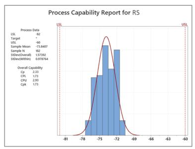
Figure 14 – Capability Analysis corresponding to RS
