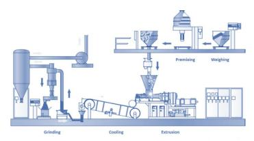
Figure 12 - Productive process scheme (FreiLacke, accessed 10 january 2020)
