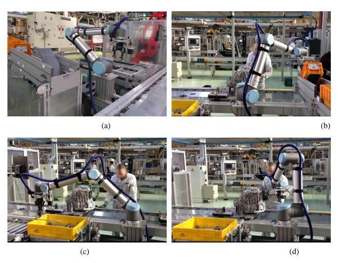
Figure 1 – Sequence of operations of the parking pawl assembly task: (a) Components setup; (b) Screws feeding; (c) Pawl feeding; (d) Pawl screwing.
