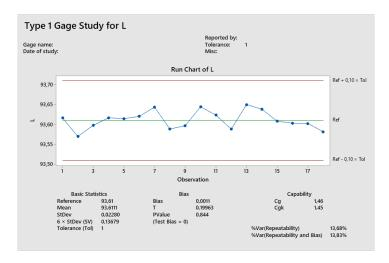
Figure 14 - Results of Type 1 Gage Study for L\*coordinate of a sample of product B
