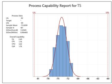
Figure 13 – Capability Analysis corresponding to TS
