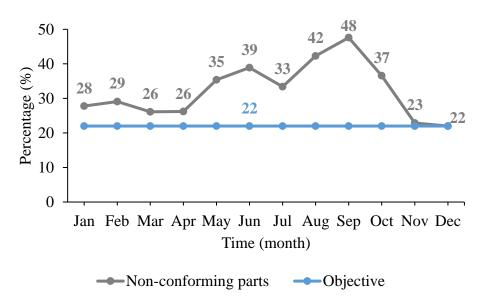
Figure 6 – Percentage of non-conforming parts in the High Gloss Blend component in 2019. Source: Internal data of Fehst Componentes, Lda, 2019.
